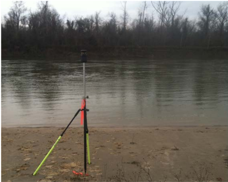
Image 14: Cross-sectional survey being performed with robotic total station at Site 080075
