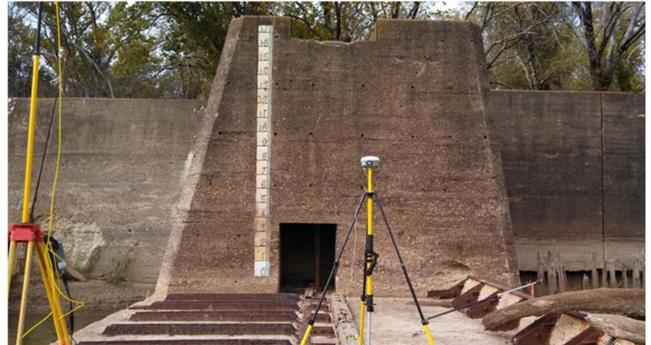
Image 10: RTK GPS base station setup at relic lock near 080444
