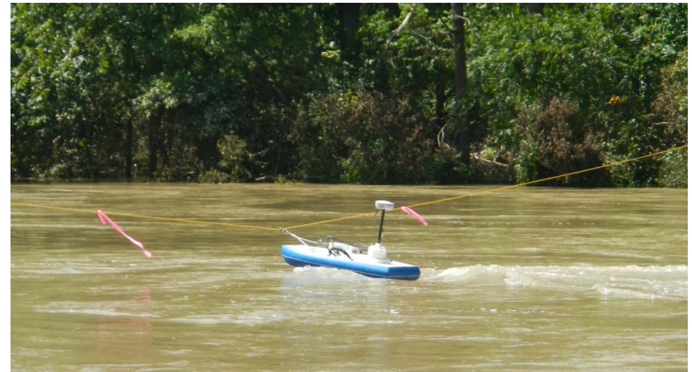
Image 13: Moving bed calculations being performed by acoustic Doppler profiler during high flows at site 080295. Similar methods are employed to calculate flow (Q) data.
