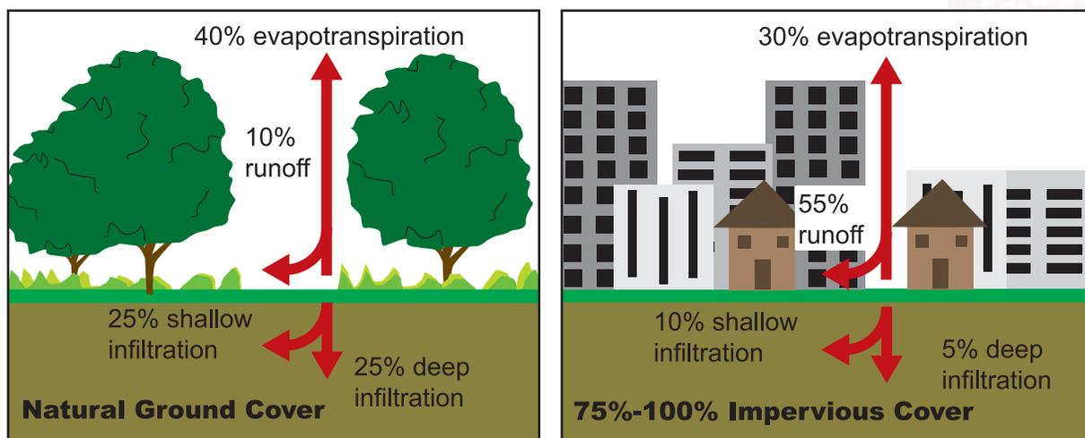
**Figure 1.** Relationship between impervious cover and surface runoff. Impervious cover in a watershed results in increased surface runoff. As little as 10 percent impervious cover in a watershed can result in water-quality problems. (Source: USEPA)
